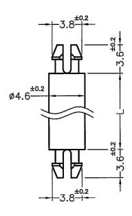
MOUNTING HOLE Ø3.2 THICKNESS 1.6mm
