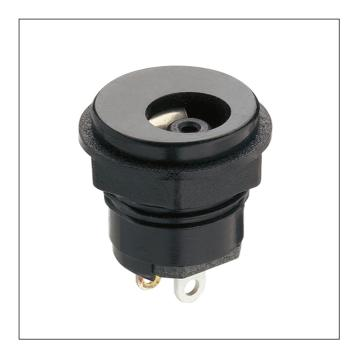
Power supply chassis socket acc. to JEITA RC-5320A JSBJ5, straight version, with break contact and solder eyes, for front side mounting
