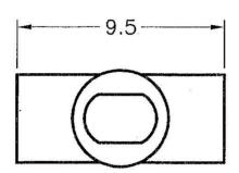
HOLE IN P.C.B Ø2.5 P.C.B THICKNESS 1.6
