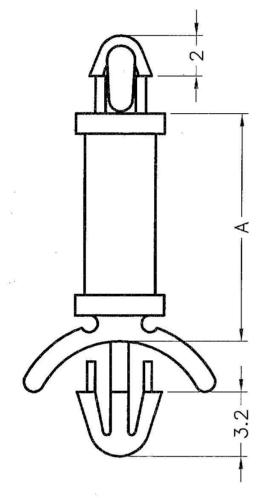
HOLE IN CHASSIS:03~03.2 CHASSIS THICKNESS:0.8~2.0
