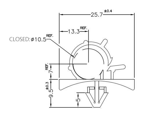
HOLE IN CHASSIS: Ø6.5 CHASSIS THICKNESS: 0.8~1.6
