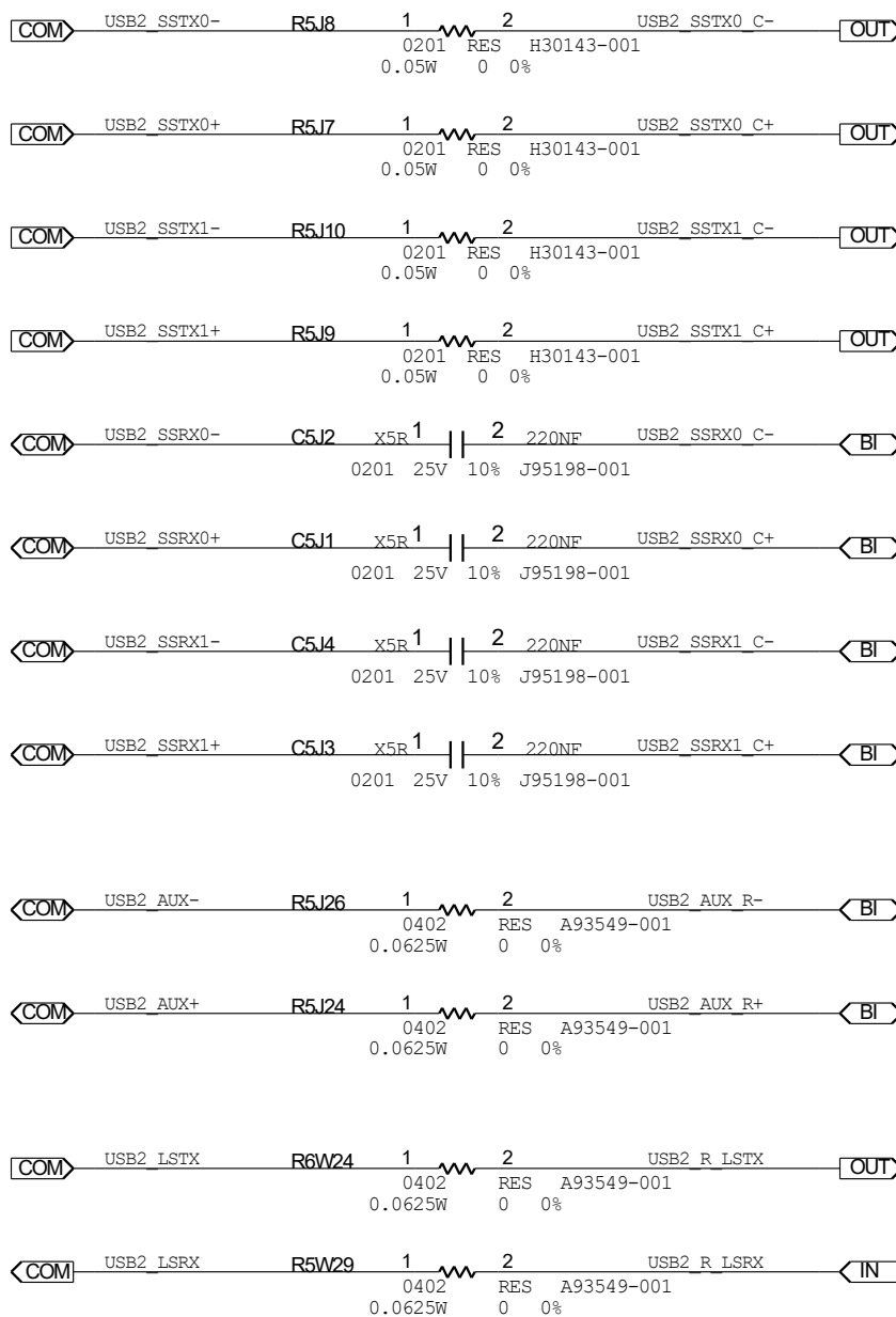
Figure 36: USB4 on COM-HPC USB Port 2 (Fig 1 of 6): COM-HPC Side RX Coupling Caps
