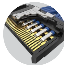
Two rows of high-density contacts directly soldered to the cable
