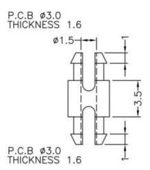
All measurement does not include gate which raises under 0.3mm.
