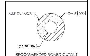
JNLESS OTHERWISE SPECIFIED DIMENSIONS ARE IN MILLIMETERS TOLERANCES ARE: **DECIMALS** ANGLES X.X: ±0.3 [.01] X.XX: ±0.13 [.005]
